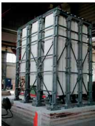
Heavy-load constructions made of AnnaSicon® 25 for hang firing of rollers
