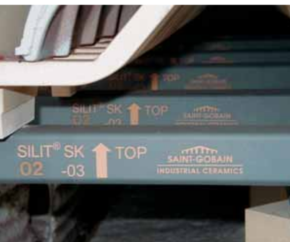
Beams out of Silit® SK and AnnaSicon® RT for firing roof tiles
