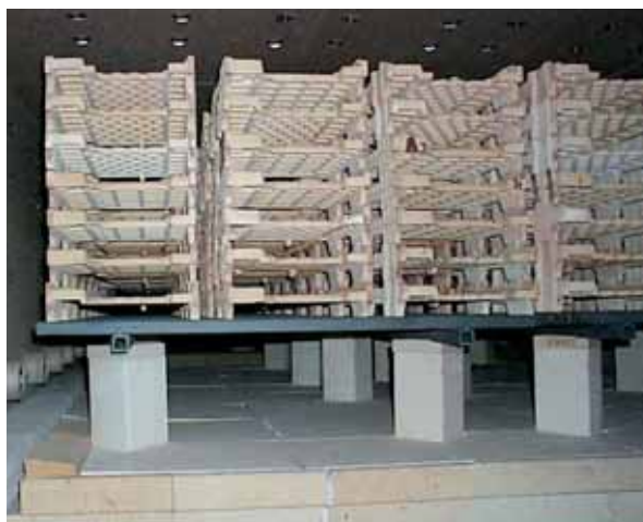
Beams out of Silit® SK and AnnaSicon® RT for firing roof tiles
