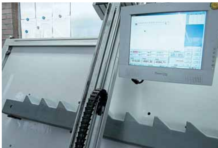
Numeric controlled measuring device for complex components
