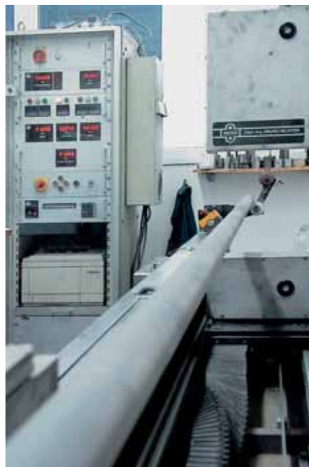
Laser test equipment for rollers (Deflection/Bending)
